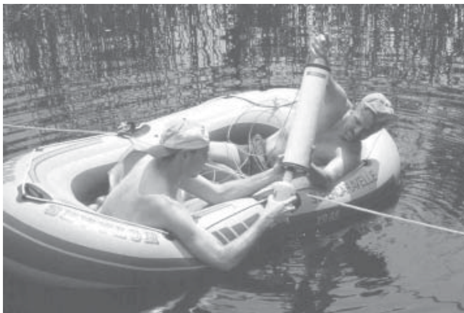
Obtaining water sample with Kemmerer Bottle at Stafford's Creek Blue Hole, Andros Island, Bahamas (photo by H. Hobbs III).
